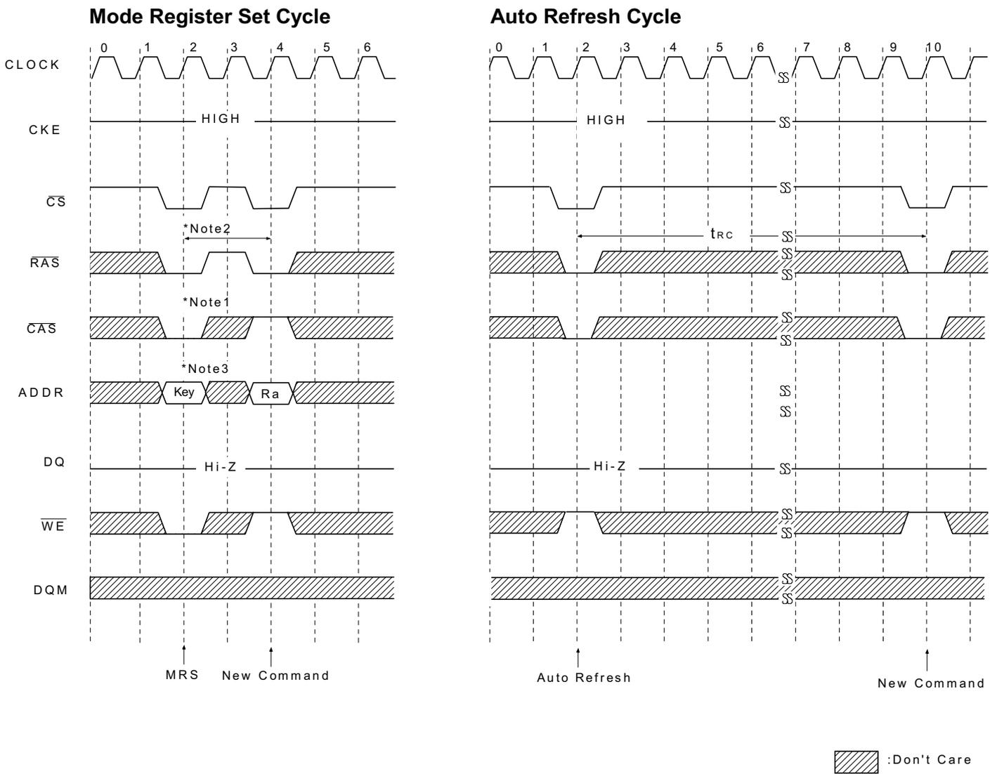
\*Both banks precharge should be completed before Mode Register Set cycle and auto refresh cycle.
