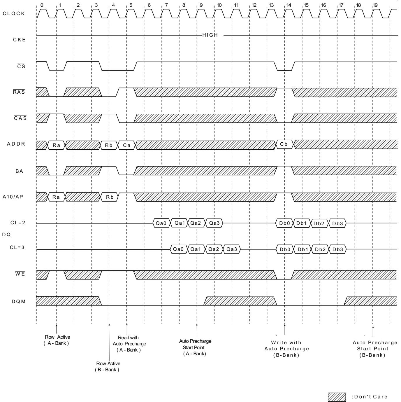
\*Note: 1.t<sub>CDL</sub> Should be controlled to meet minimum t<sub>RAS</sub> before internal precharge start
