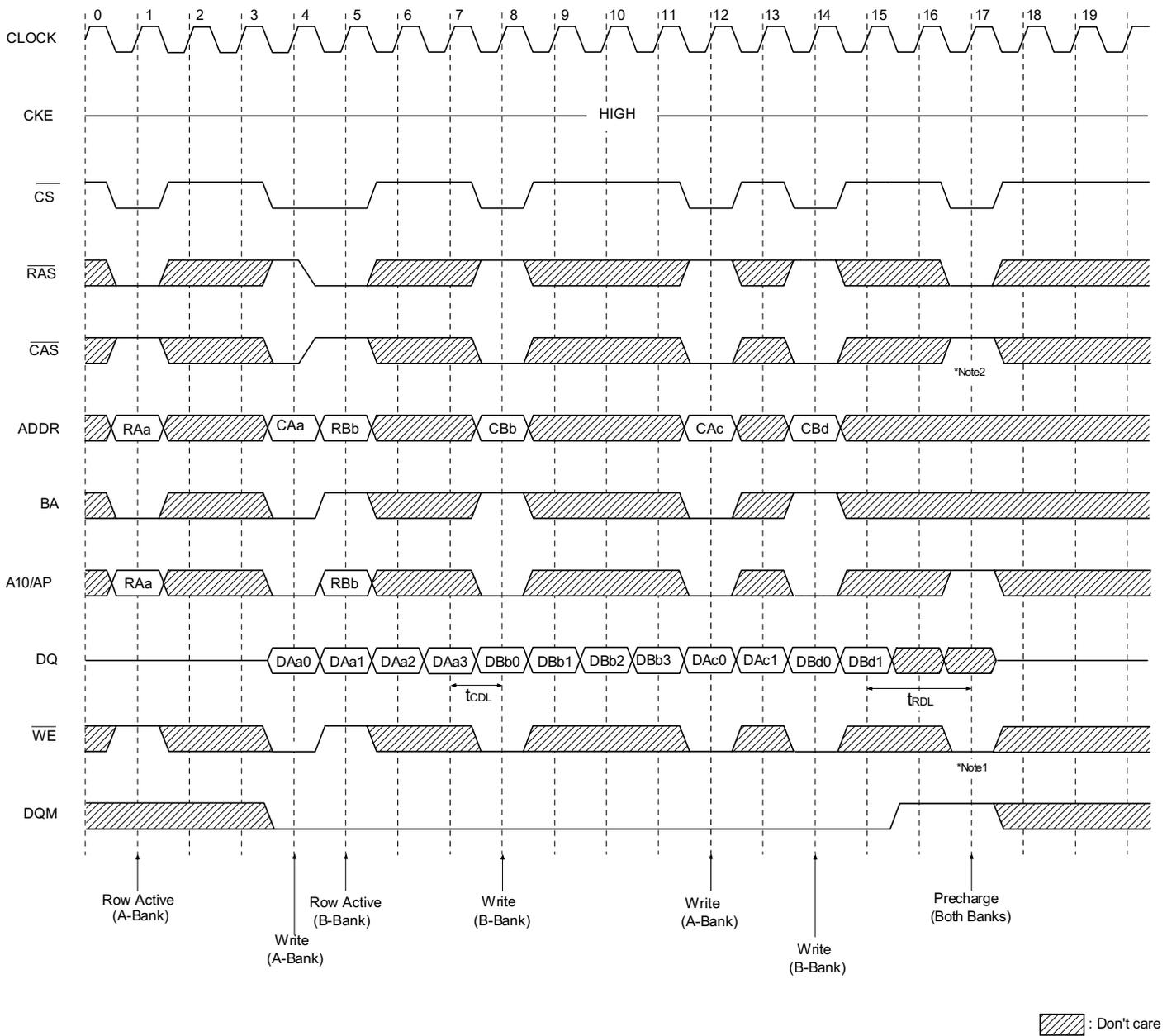
\*Note: 1. To interrupt burst write by Row precharge, DQM should be asserted to mask invalid input data.
