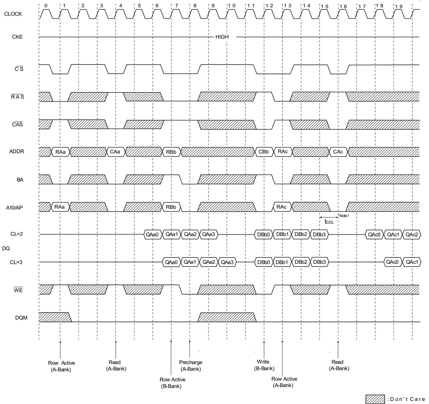
\*Note: 1.  $t_{CDL}$  should be met to complete write.
