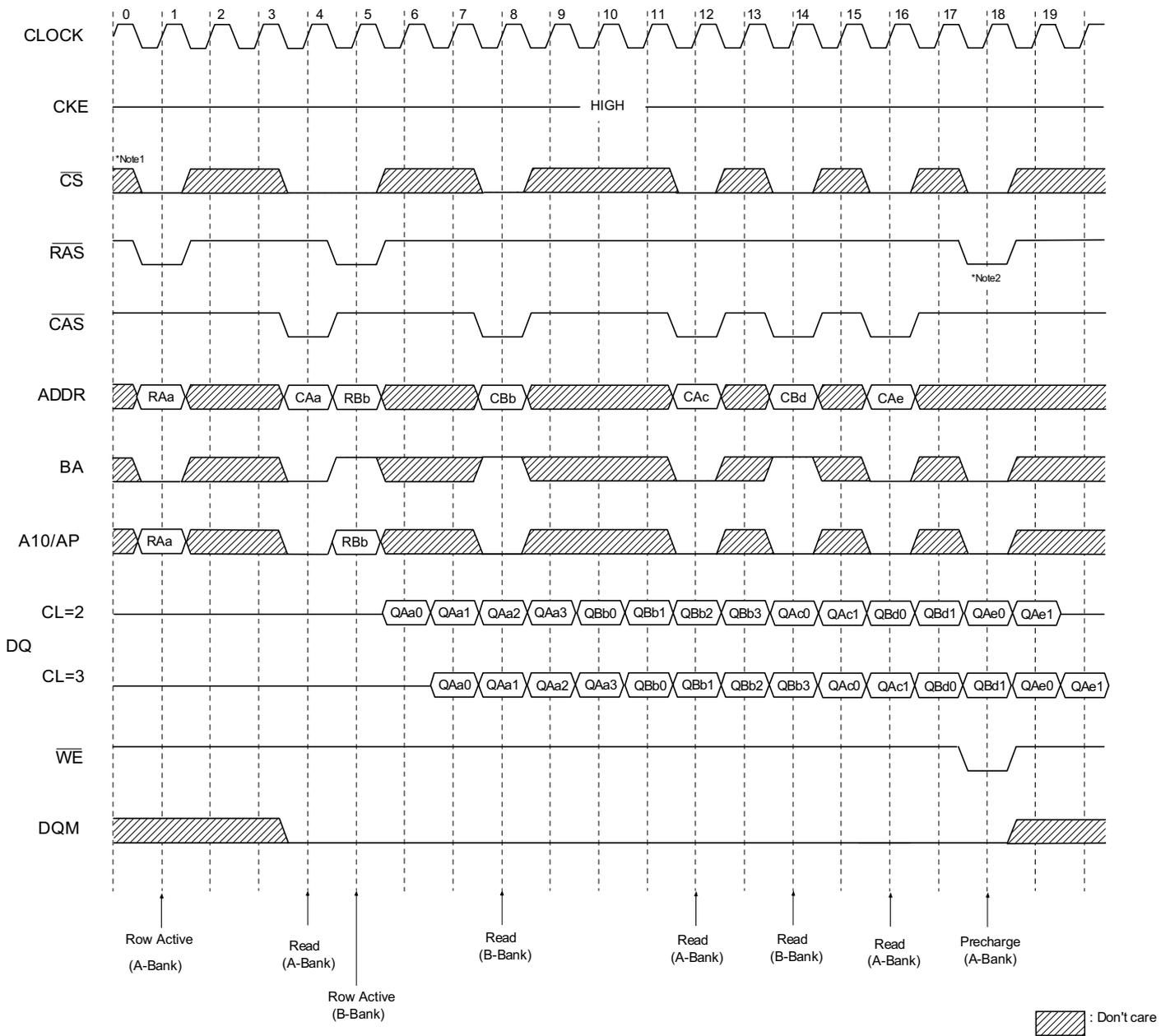
\*Note: 1.  $\overline{CS}$  can be don't cared when  $\overline{RAS}$ ,  $\overline{CAS}$  and  $\overline{WE}$  are high at the clock high going dege.
