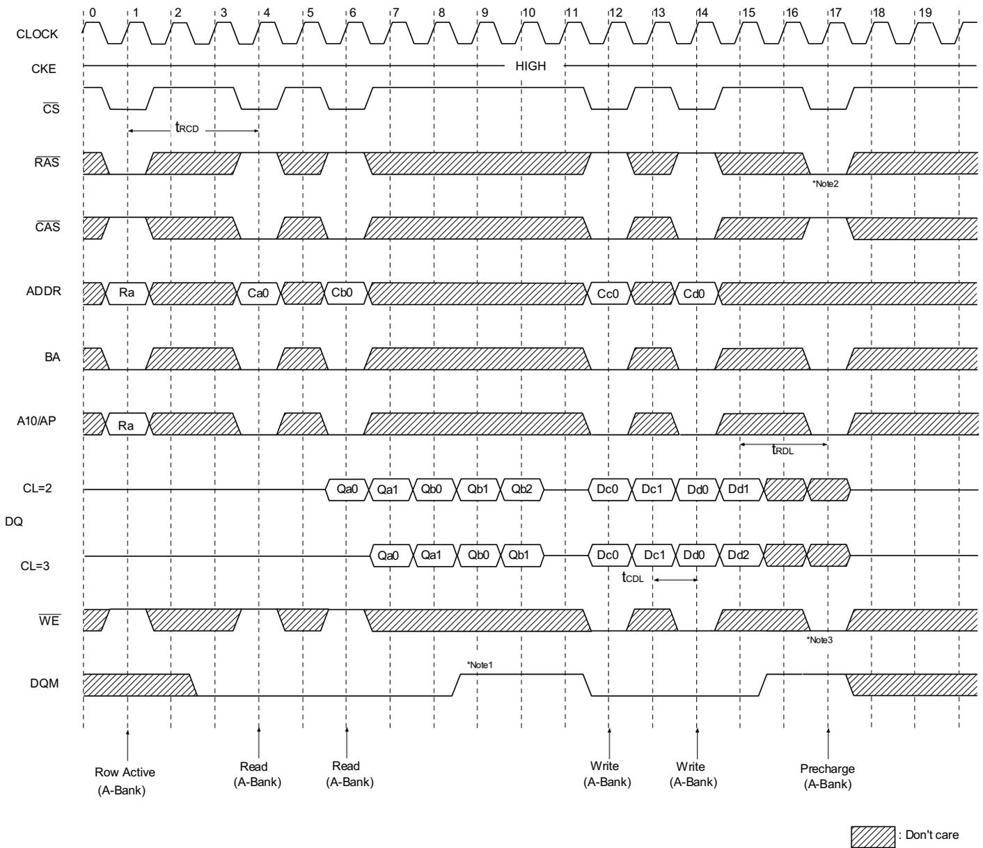
**\*Note** :1.To write data before burst read ends, DQM should be asserted three cycle prior to write command to avoid bus contention.
