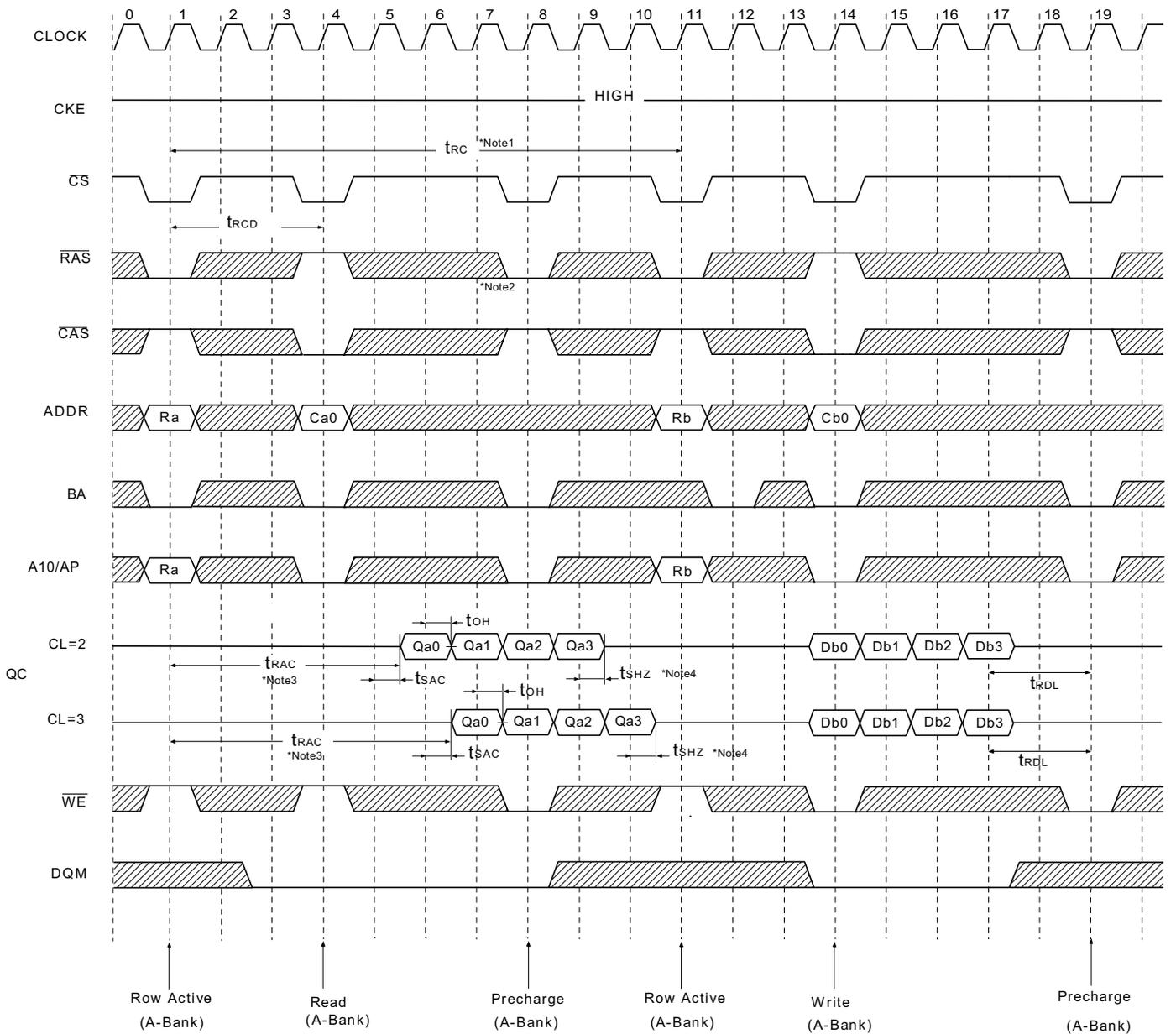
**\*Note:** 1. Minimum row cycle times is required to complete internal DRAM operation.
